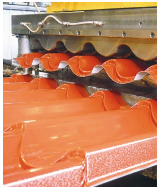
Beckry® Tough derives its surface texture from the incorporation of polymeric beads in the paint formulation.
