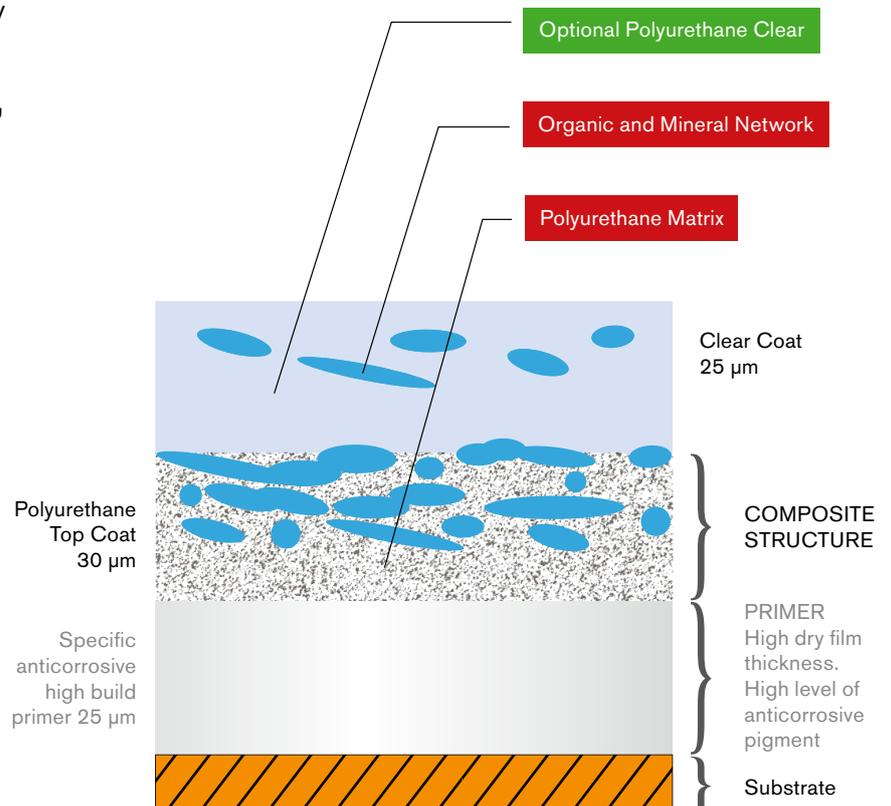
**Beckry®Tex PUR** is a topcoat based on polyurethane resin that offers a very high outdoor durability and makes it possible to achieve high dry film thickness. It gets a textured surface when cured and contains polyamide giving the surface a very good scratch and wear resistance. Beckry®Tex PUR has excellent colour and gloss retention as well as chemical resistance. It is recommended to be used in conjunction with the high build polyurethane primer **Beckry®Prim**.
