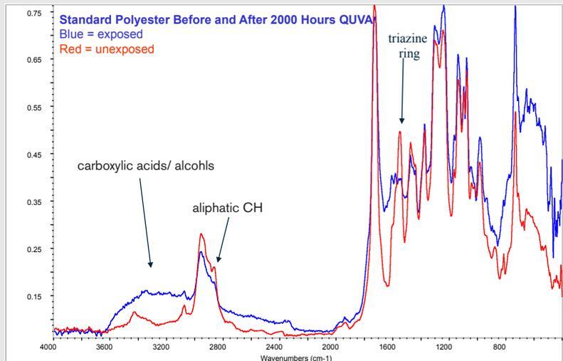
**Figure 3** IR spectra of polyester melamine system in different environments
