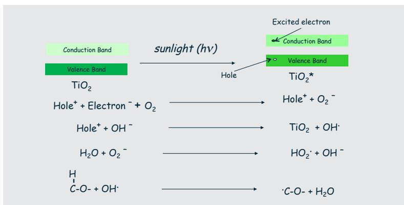
Figure 2 Attack of TiO<sub>2</sub> generated radical on alpha hydrogen
