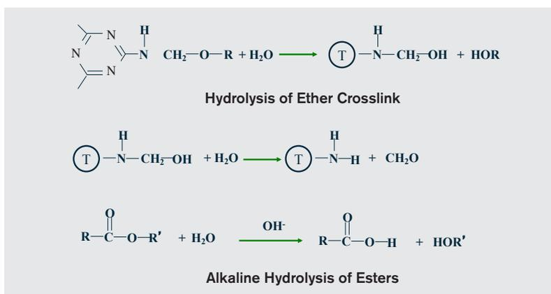
Figure 1 b Hydrolysis of melamine and ester linkages
