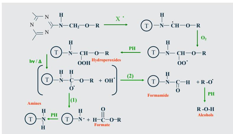
Figure 1a Mechanisms of degradation by photo-oxidation of melamine linkages
