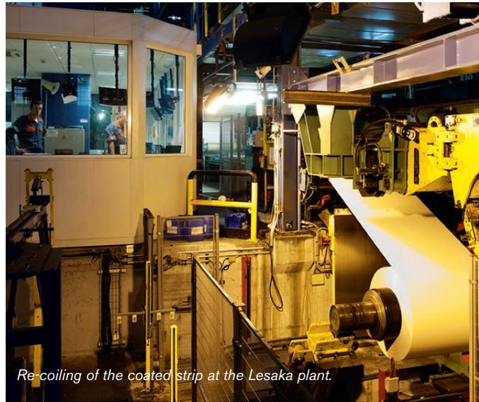
*Re-coiling of the coated strip at the Lesaka plant.*
