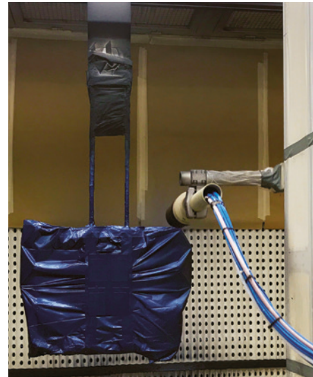
The high-speed bell applicator in action in the Industrial Coatings lab at Beckers Sweden
