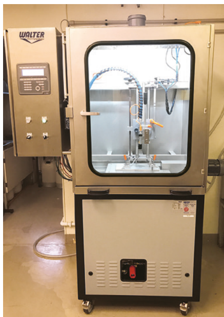
The high-pressure wash unit in the Industrial Coatings lab at Beckers Sweden
