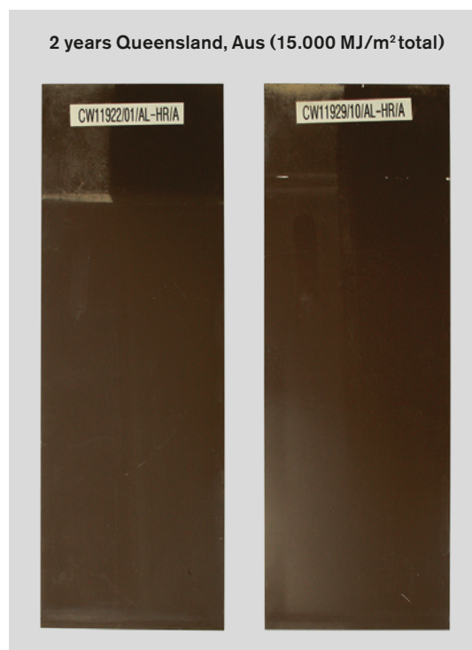
Figure 1: degradation characteristics of Beckry®Tech 2001
