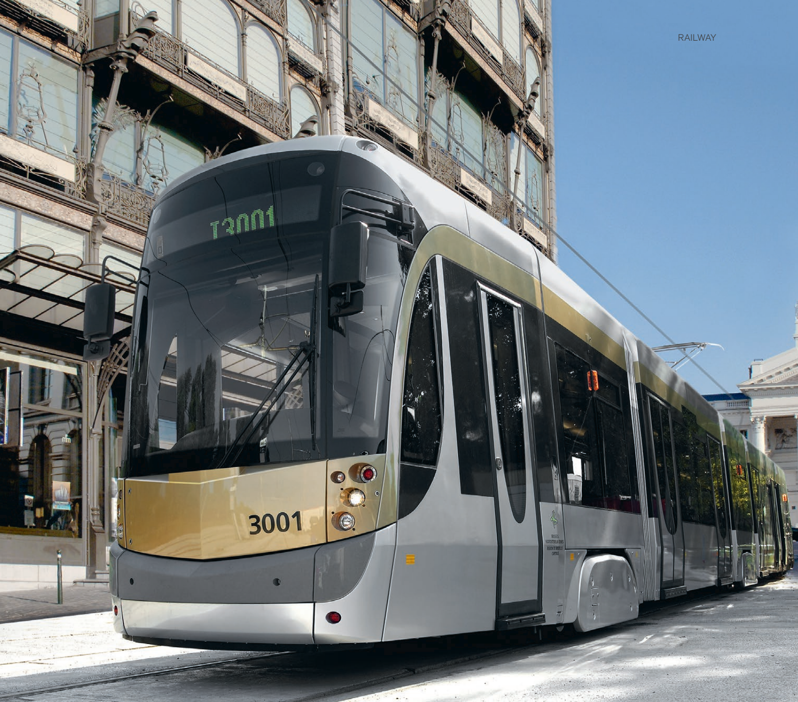
The Bombardier FLEXITY Outlook low-floor tram operated by STIB-MIVB (the Brussels Intercommunal Transport Company). The tram is finished in a five-layer fully waterborne Beckers paint system.
