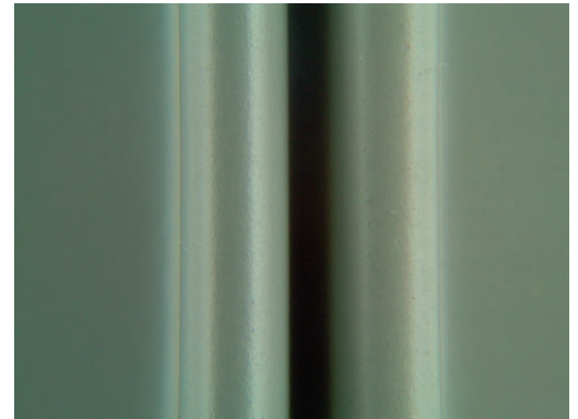
Figure 6: 2.5T Bend on Backing Coats Bio Based RHS.
